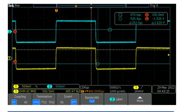
Balanced Line Level square wave response with input fed through 10k 14 dB resistive attenuator
