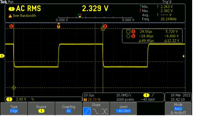
Square wave response at 20 kHz is clean with no overshoot (note: this is into a purely resistive load)
