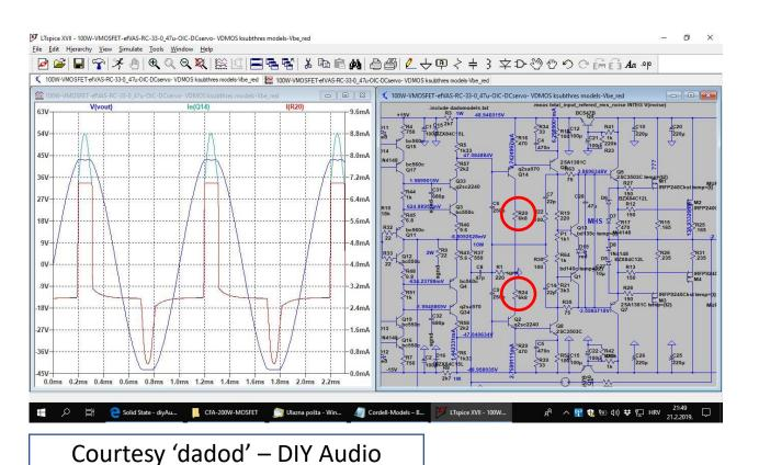
In this technique, R20 and R24 limit the maximum amount of current that can be injected to the base of the main VAS transistors Q6 and Q8 by causing the beta-enhancer stage Vce≈ 0 when overdriven.
