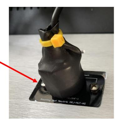
Attention: the headphone socket mounting nut must be ordered separately. The Mouser Pt# is NRJ-NUT-MS.
