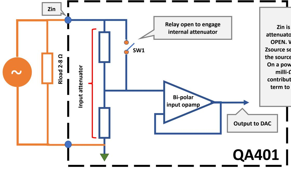
The input attenuator is high impedance and therefore contributes a significant thermal (Johnson) noise term to the measurements. The internal QA401 20 dB attenuator raises the noise floor by about 30 dB. Mains noise components are therefore buried beneath the instruments noise floor which sits at about -100 dBV vs -135 dBV (typical power amp measurements with the power OFF)
