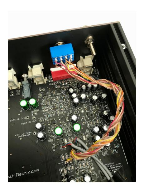
Here is a picture of my first build (I did 2 builds). For the wires between the switch and the PCB, I used ribbon cable. This wiring is probably suboptimal and should have been twisted a bit more and run closer to the edge of the RHS panel to reduce to opportunity for noise pickup.
