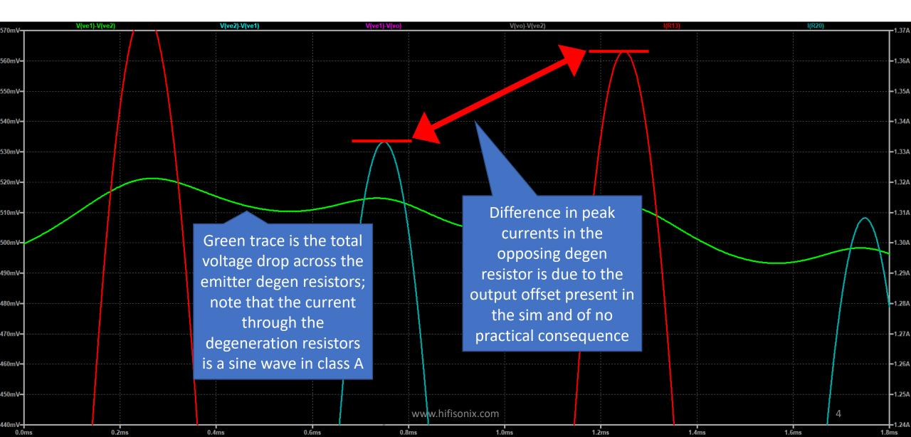
We go back to slide 1 but zoom into the differential voltage across the emitter degen resistors – this is the green trace below with C17 = 100uF (vs 0uF in the design)
