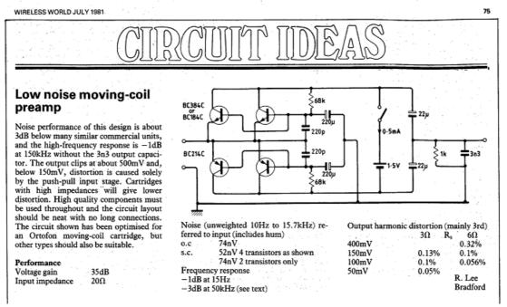
A version using Hitachi 2SA1084 / 2SC2546 and running about 3mA is probably the **lowest noise** such device in the known universe. 3dB NF for 5R source. Less than 40nV over 20kHz. ie <0.28nV/rtHz
