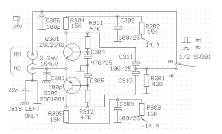
This, the most successful powered version, overcomes the main disadvantage of the battery circuit; that the gain goes down and noise goes up as it runs down. But at 0.5mA, a C size R14 alkaline lasts for months before you notice any deterioration. And this more complex version may put current through the input. (in practice not a problem for MC cartridges)
