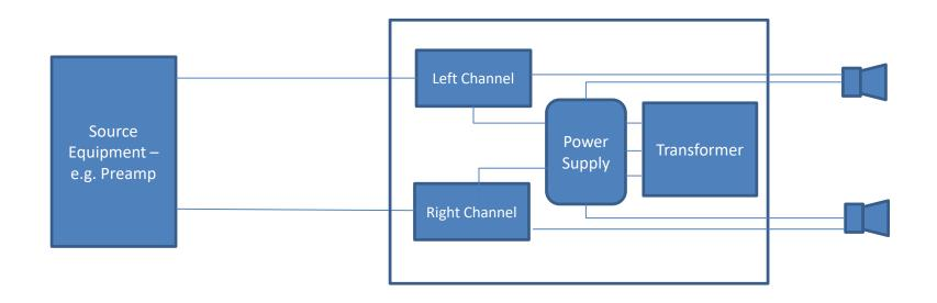
A source on the left provides inputs to an amplifier on the right. For clarity, the interconnections are simply shown as single lines (this is why we call it a *line diagram*) – they would in reality consist of a signal and a return (normally the cable shield). Inside the amplifier we have the left and right power amplifiers themselves, and a power supply – usually a bank of reservoir capacitors and associated rectifiers and a transformer.
