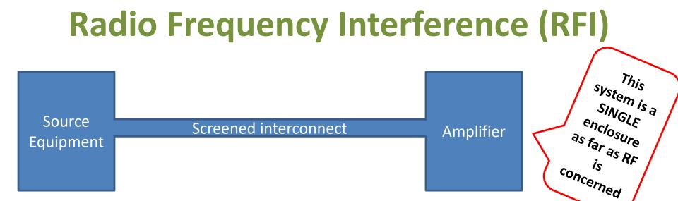
The shielded interconnect works extremely well at RF because the shield works to block the RF EM field and in doing so effectively makes the source equipment, the amplifier and the shielded cable one enclosure – and this is one of the keys to ensuring RFI immunity.
