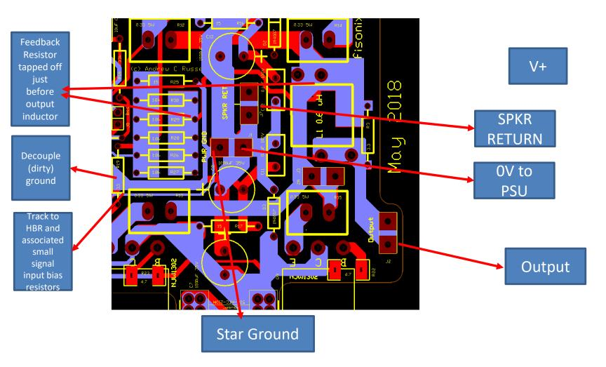
Here is a close up of the connections around the STAR GROUND on the PCB. The small signal ground connects directly to the OV terminal and the decouple grounds connect at that point as well. The speaker return joins at the OV and there are no other connections between it and the OV terminal. <u>The STAR ground on the PCB is the ground reference point for the whole amplifier</u>
