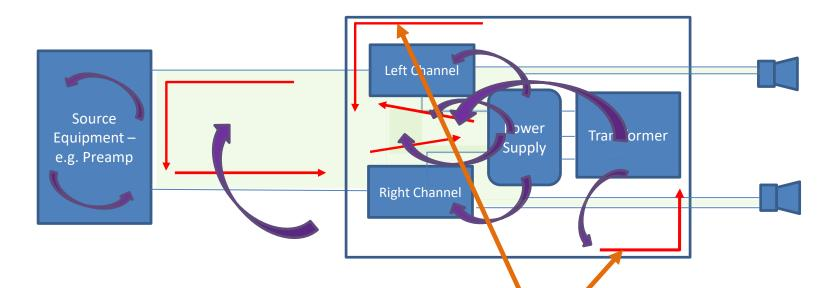
In this final example, we show the internal stray magnetic fields impinging on the metal housing of the amplifier, causing noise currents to flow in the metalwork. For this reason there should only ever be **one and only one connection between the electronics OV and the housing** – if you have more than one connection, you run the risk of creating a loop and injecting unwanted noise into your circuit.
