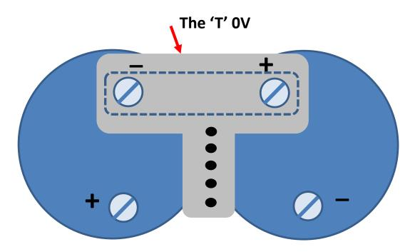
This drawing shows how you can minimize the loop area in the vicinity of the main reservoir caps by 'folding' the capacitors so that the + and – are closer than shown in the previous two diagrams. There are very large charging currents flowing into the reservoir capacitors, and they therefore radiate significant EM fields. Keep small signal wiring away from your reservoir capacitors. Make sure you keep the capacitors as close together as practically possible.
