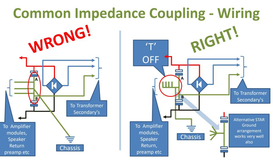
On the right hand side we see how to do it correctly. 'T' off from the OV junction where the two reservoir capacitors are connected. Then make the connection to the chassis, and after this the connections to the amplifier modules and small signal circuits. How these latter connections are ordered can also impact noise and distortion – we'll look at this next .
