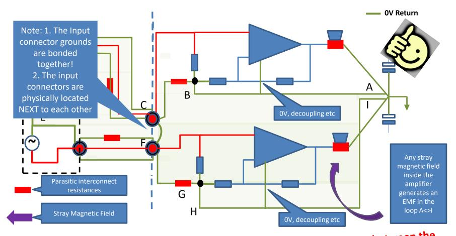
Keep the areas shaded GREEN both <u>inside the equipment</u> and externally between the interconnect cables as small as possible to minimize the total loop area! Bond the Left and right input signal grounds together; mount the input connectors NEXT TO Next, we will show how Hum Breaking Resistors (HBR) help
