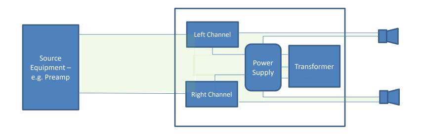
Highlighted in this example is the total loop area. Note that it extends out between the equipment, and between the internal signal interconnects, power supply wiring and to the speakers
