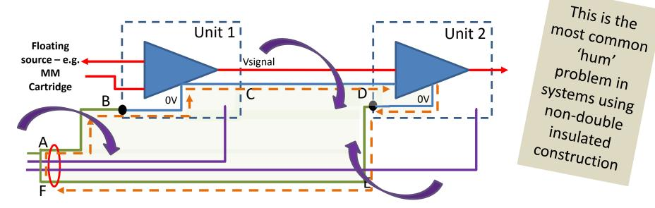
Any magnetic field impinging on this loop (the green area) will generate an EMF and cause a current to flow around the loop A>B>C>D>E>F>A i.e. an EARTH [GROUND] LOOP CURENT
