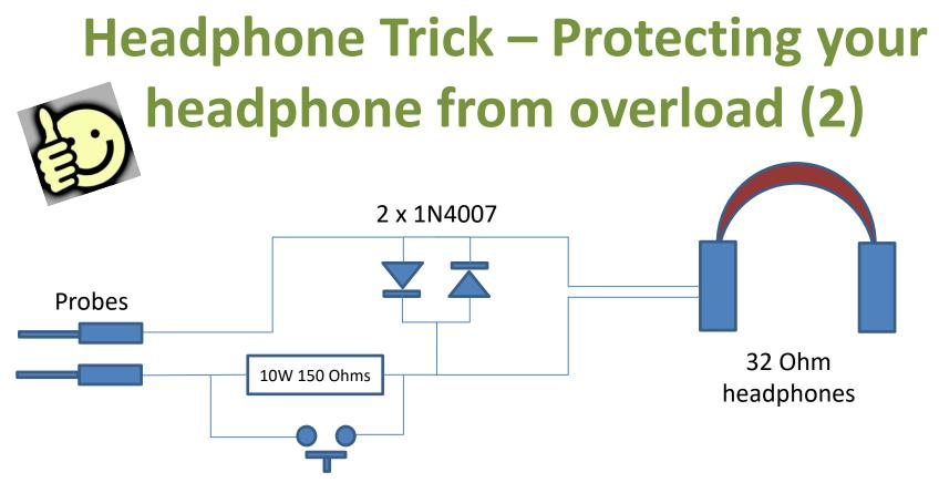
Connect the headphone probe across the amplifier output terminals.
