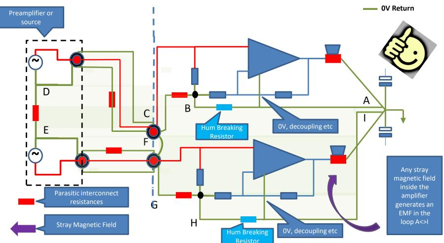
To reduce the error voltages appearing across the parasitic interconnect and ground resistances, the loop current must be reduced. This is accomplished using 'Hum Breaking Resistors' (HBR). This reduces the loop current and forms a voltage divider with the parasitic resistors. For example, if the parasitic resistances total 1 Ohm and the HBR is 10 Ohms, the reduction in cross channel ground loop noise is in the order of 20 dB.
