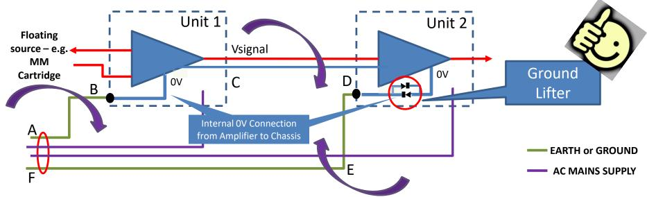
The ground lifter consists of two diodes placed in 'anti-parallel' between the amplifier power supply OV and the chassis (WHICH MUST BE EARTHED/GROUNDED) and BREAKS THE GROUND LOOP so no ground loop current can flow between C and D
