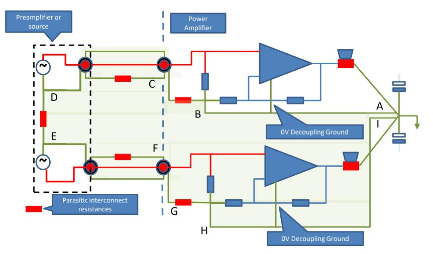
The shaded **GREEN** areas represent the total loop area between the two pieces of equipment wrt the cross channel ground loop. *Note carefully that the loop area includes the areas inside the preamplifier and power amplifier*. Next, we will consider what happens in the presence of magnetic fields . . .
