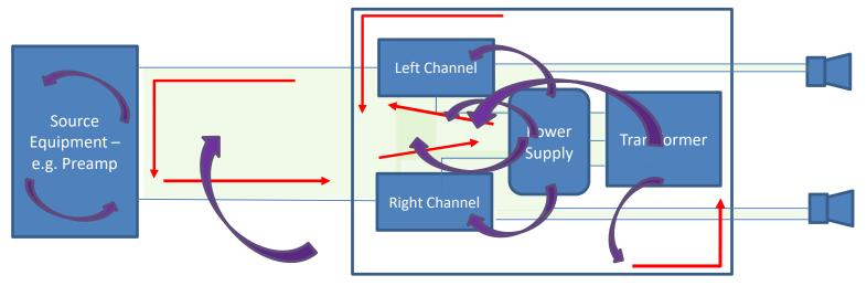
Stray magnetic fields impinging on the green shaded areas shown above drive signal currents (i.e. noise) at the source frequency. These create loop currents that degrade signal to noise ratios if they are allowed to combine with the signal. There are many potential loops and stray (unwanted) magnetic fields in an amplifier – we have touched on only a few here.
