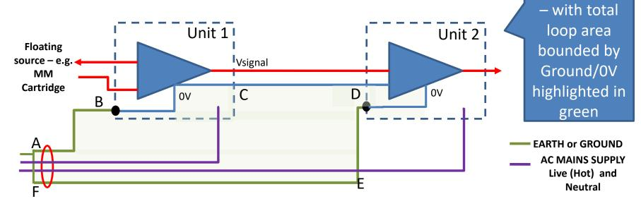
In this line diagram, the electromagnetic loop is the TOTAL AREA prescribed by A>B>C>D>E>F>A shown in light green. It is important to note that the loop is bounded by the signal return connection (C to D) between the two pieces of equipment and the safety earth [ground] which is the GREEN wire.
