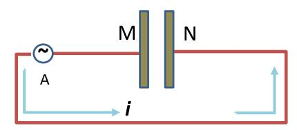
In *capacitive* coupling, source A causes and *electric field* across M and N (i.e. the capacitance that exists between two parts of a circuit) that drives a *displacement current i* that flows around the circuit. When M is positive with respect to N, electrons flow around the circuit to N. When M is negative with respect to N, electrons are repelled and flow away from N towards the source.
