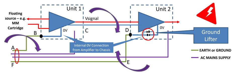
It is IMPORTANT that HIGH POWER rectifiers are used – use a chassis mount 25-35A device with a surge rating of >200 Amps
