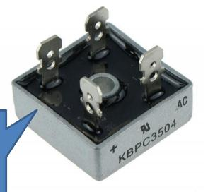
**35A 400V** or higher voltage Bridge Rectifier e.g. <u>KBPC3504</u> This must conduct the FULL fault current until the RCD/GFCI trips at the mains distribution box. The currents can range from 10 to 150A for at least 1 mains cycle, but can be 2-3 mains cycles. The peak single cycle surge current capability of this particular bridge rectifier is 400 Amps
