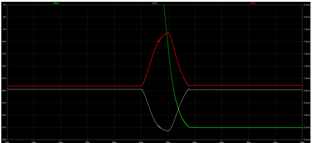
Figure 9 - DB response to worst case audio step signal with 400kHz input bandwidth limiting filter
