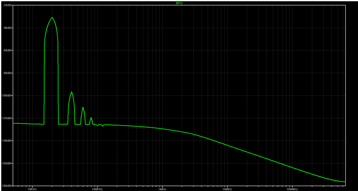
Figure 5 – A simulation of the power rail harmonics of the class A gain block (10V pk into 300 \Omega at 20kHz)
