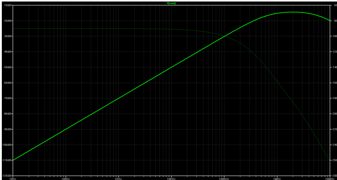
Figure 2 - Just 5 pF of coupling means at 10 kHz, noise performance is degraded to -50 dB with 1k + 10k feedback resistors (gain of 11)
