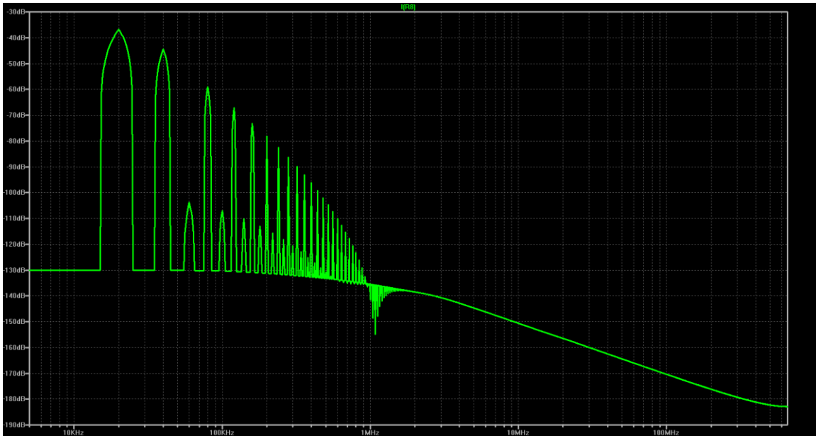
Figure 6 – Simulation of Class AB Operation Supply Rail Harmonics (20 kHz @ 10V pk into 300 \Omega with 3mA OPS bias current). The lower order harmonics are in the 100 to 300uA range.
