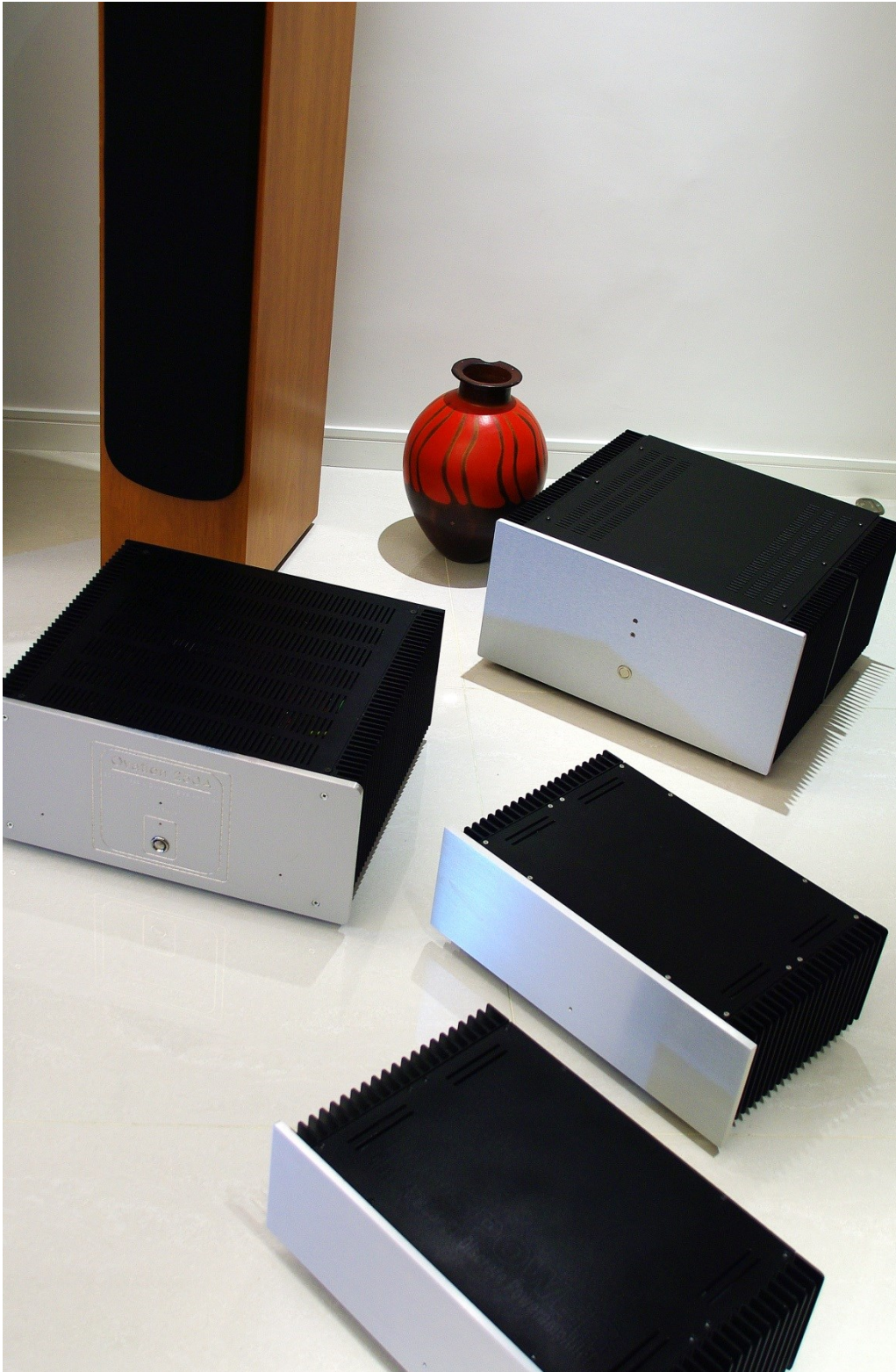
Hifisonix amplifiers from front to rear: 100 W class AB CFA nx-Amplifier, 15 W CFA Class A sx-Amplifier; Rear LHS 280 W class AB VFA Ovation 250 and rear RHS the 180 W class AB VFA e-Amp
