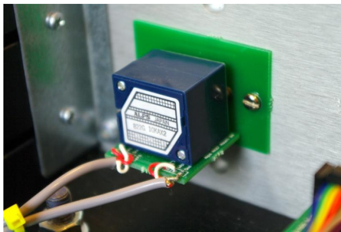
Figure 19 - Volume Control Mounting Detail
