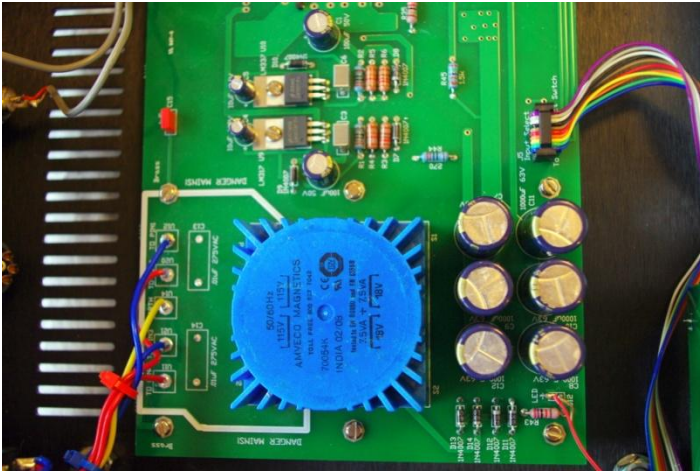
Figure 2 – View of the Power Supply Section
