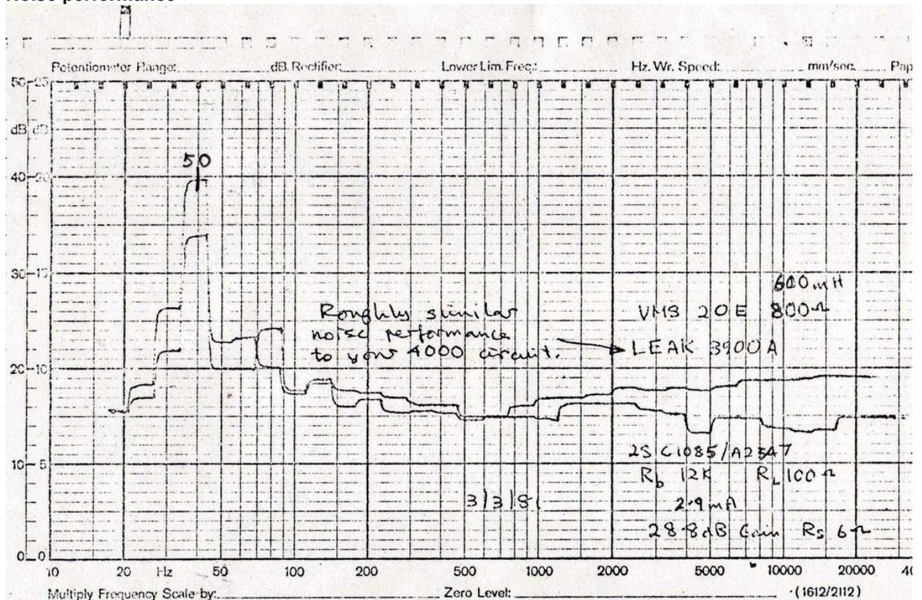
Here's a 1/3 8ve noise plot. The B&K 2307 chart recorder has slipped by 1 tooth so 50Hz (hum) appears at 40Hz. 1dB/division
