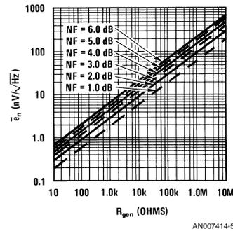
FIGURE 5. Spot NF vs  $R_{gen}$  when Considering Only  $\bar{e}_n$  and  $\bar{e}_R$  (not valid when  $i_n R_{gen}$  is significant)
