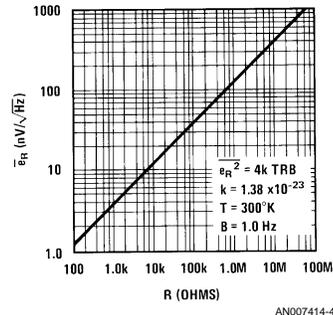
FIGURE 4. Thermal Noise of Resistor
