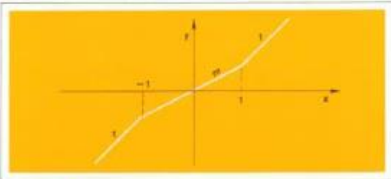
Fig. 8. Transfer characteristic of entire nonlinear stage.
