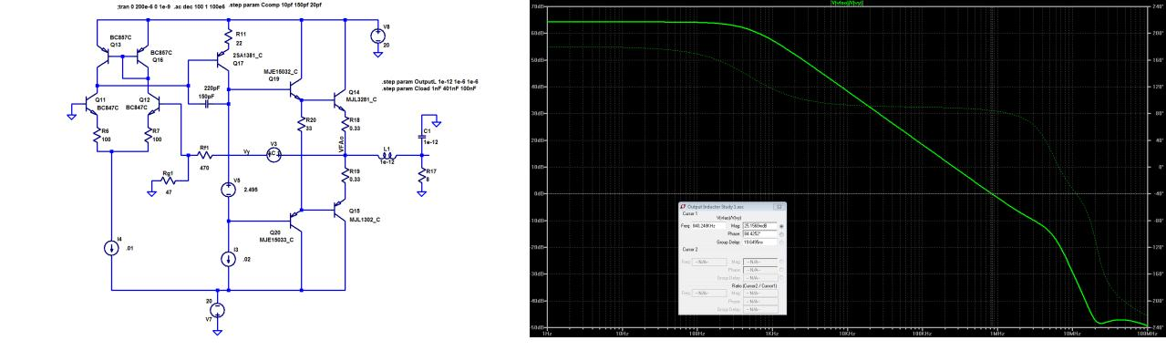
*Model Amplifier Used for this Investigation.* This is the basic amplifier design loop performance driving a standard 8 Ohm load with the capacitive load set to ~0 F and output coupling inductor set to 0
