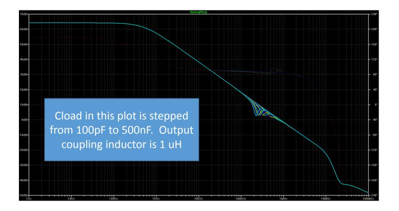
**1uH is Enough to Ensure Unconditional Stability.** In this plot, Ccomp1 is set to 150pF, setting the ULGF to ~840 kHz. A 1uH inductor is used to couple the amplifier to the output load. The result is the amplifier is unconditionally stable for loads of up to 500nF. The gain and phase margin are hardly affected by the capacitive load.
